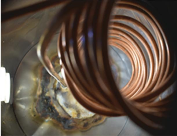
Figure 5. The heat exchanger (coil exchanger).
